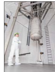
The titanium cryostat that encloses the LUX dark-matter detector, seen here suspended in its water tank. (Image credit: Matt Kapust/Sanford Underground Research Facility.)
