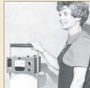
A small, just about portable, radiation detector, known as the Albatros I Neutron Monitor, has been designed by the Radiation Physics section at Batavia to monitor fast neutrons, which are usually the most serious radiation hazard in personnel-occupied areas when a high-energy accelerator is operating (in certain areas high-energy muons may also be a problem, but for most areas neutrons are the most troublesome). The meter can be read in dose rate or in occupation time per day. The total integrated neutron dose is also recorded. An audible signal sounds when the dose rate exceeds 50 mRem/hr. The unit operates either on a battery pack or on AC power. It
