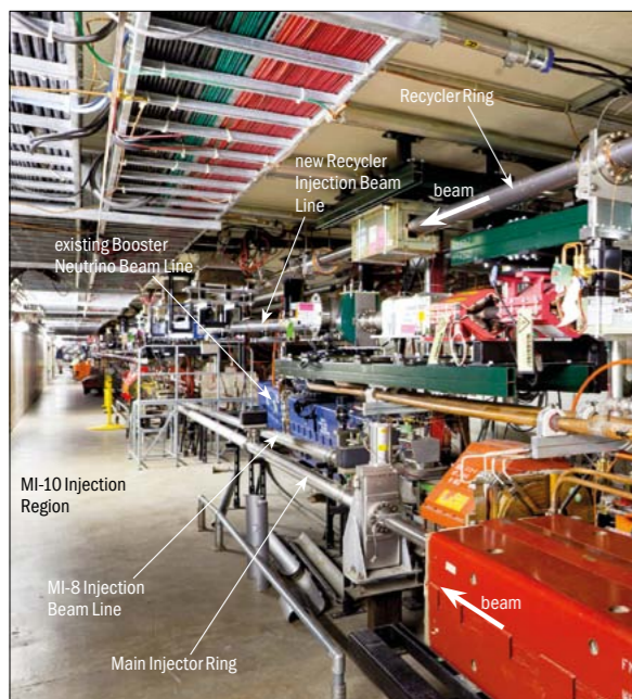
Fig. 4. The injection area showing the Main Injector (MI), the Recycler, the Booster Neutrino Beam, the MI-8 line and the Recycler Injection line. (Image credit: Marty Murphy, Fermilab.)
